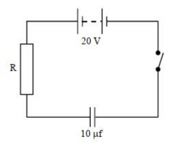
A capacitor of capacitance 10  $\mu$ F is fully charged through a resistor R to a p.d. of 20 V using the circuit shown. Which one of the following statements is **incorrect?**
